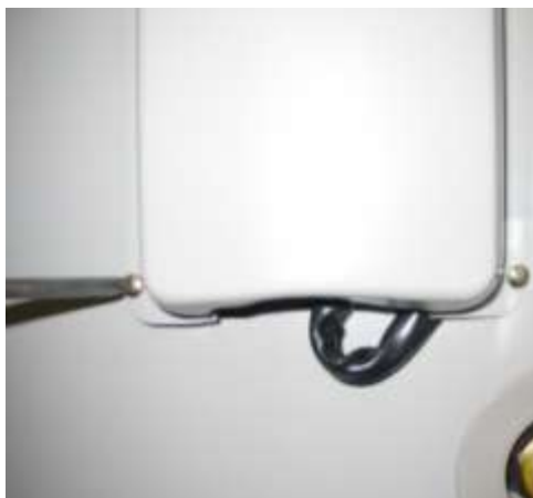
Step 2 remove screws from lower front cover
