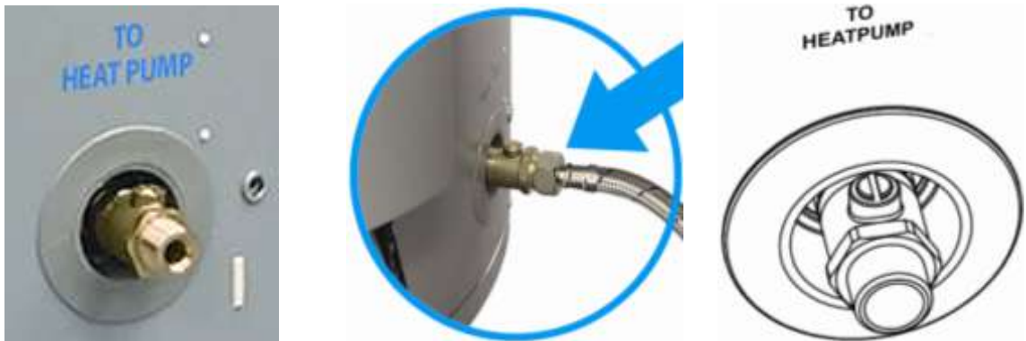
Step 15 attach flexible hose with blue stripe to inlet and ball valve in open position
