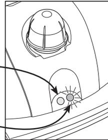
Once Boiler is filled and the green Steam Ready Indicator Light glows, Steamer is ready to clean.
