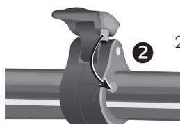
2. Line up the peg on Locking Clamp with the hole on Extension Tube and...
