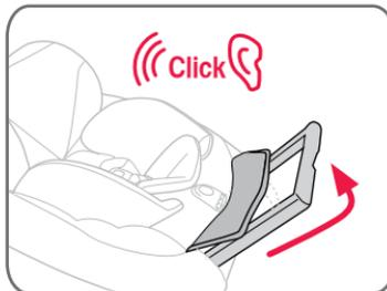
Locate the stabilising bar under the front flap of the cover. Lift the flap at the end of the seat to sufficiently access the stabilising bar. Pull out the stabilising bar fully and then gently push toward the headrest until you hear a click. The stabilising bar is now locked in place.
