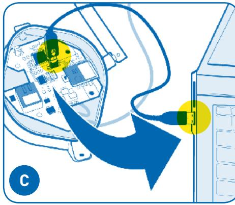
Attach the iAquaLink device to an internet connected PC or Mac® with a USB cable.
