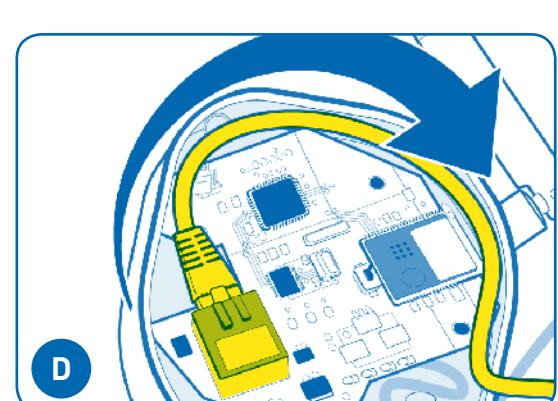
Wrap the cable as shown inside the device and use the break-away as an exit hole. Replace the rubber gasket & cover.
