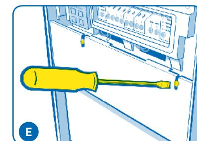
Reassemble the power center, making sure no wires are pinched. Replace all panels or screws before returning electrical power to the power center.
