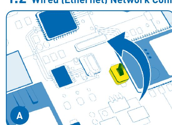
Remove the device lid by removing the two screws. Locate the WiFi/WIRED switch and ensure it is in the WIRED position.
