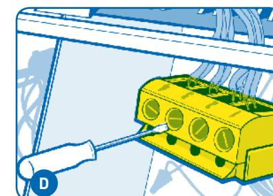
Up to two devices can be connected to each 4-wire connector (two wires per hole). If more capacity is needed, a 6584 multiplex board can be installed. See "helpful hints" section.
