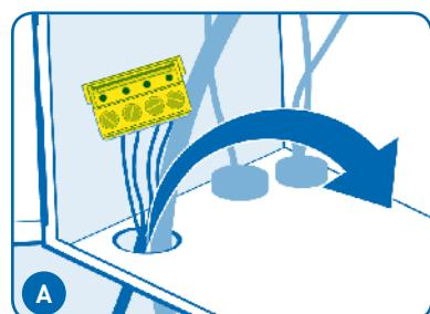
All power to the power center must be OFF! Route the 4-wire cable through the bottom access hole into the low-voltage raceway. The red 4-wire connector may not be required for all installations.
