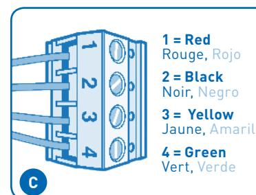
Ensure that all wires are properly attached to the red 4-wire connector. Some connectors may look different.
