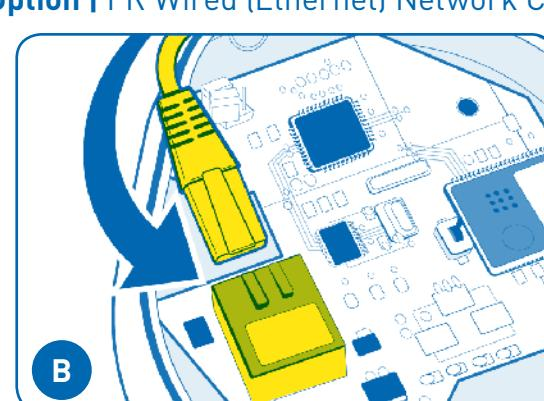
Using an Ethernet cable, connect the device to the home network's router.
