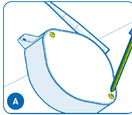
Remove the device lid by removing the two screws.
