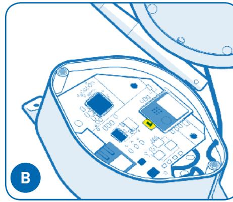
Locate the WiFi/WIRED switch and ensure it is in the WiFi position.
