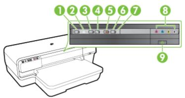
ePrint button and light Ethernet light 🚜 2 3 Wireless button (1) and light 4 Network Information button Pa 5 Cancel button X 6 Resume button and light 7 Alert light 8 Ink cartridge lights 9 Power button (1) and light
