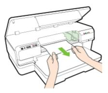
**c.** Move the carriage to the left, locate any jammed paper inside the printer on the right side of the carriage, free any paper scraps or wrinkled paper, and pull the paper towards you through the top of the printer.
