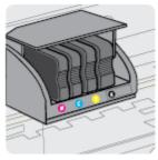
Make sure that you insert the ink cartridge into the slot that has the same colored letter as the color you are installing.
