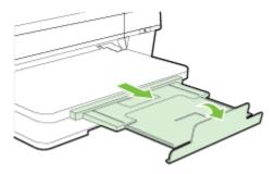
Remove excess paper from the output tray. There is a limit to the number of sheets the tray can hold.
