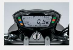
A multifunction LCD instrument panel displays gear position, digital speedometer, tachometer, as well as indicators for odometer, trip meter, average/instantaneous fuel consumption, driving range, clock, water temperature gauge and fuel gauge. Backlight is adjustable in six levels of brightness and can be set to your preference.
