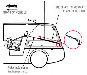
The shaded areas of this diagram illustrate the possible locations of the anchor fitting. Within each shaded area is an anchor fitting showing the correct way to install the fitting. Ensure the anchor fitting is aligned as illustrated unless stated otherwise in the vehicle owner's handbook.
