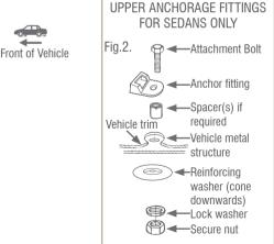
ONLY USE A 5/16 UNC GRADE 5 BOLT. IF THE BOLT IS NOT THE CORRECT LENGTH THE CAR MANUFACTURER'S HAND BOOK CAN PROVIDE ADVICE ON THE CORRECT LENGTH BOLT.
