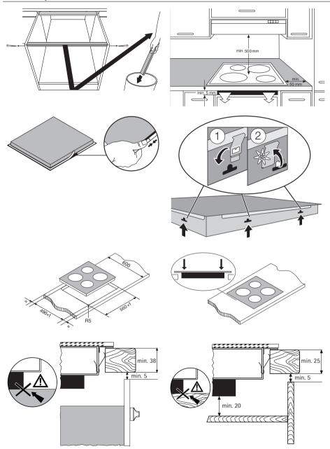
(!) Warning! Surface temperatures of base exceed 95°C, under bench access must be restricted by use of
