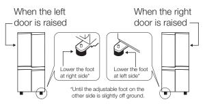
4 Remove the 4 screws from the bottom of the refrigerator and use these to fit the kickplate (supplied inside the refrigerator compartment).
