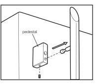
3 The pedestals can be removed from the door (if necessary). Remove the phillips head screw and pull the mounting block away from the door.
