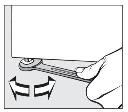
The screw feet can be adjusted to compensate for any unevenness in the floor.
