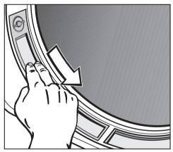
Use your fingers or a vacuum cleaner to remove the fluff from the two fluff filters in the door opening.
