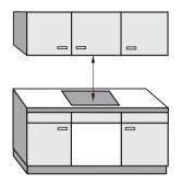
When two or more appliances are installed together below a rangehood, e.g. a gas appliance and an electric cooktop, which have different safety distances given in the installation instructions, you should select the greater distance of the two.
