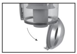
3. Ensure the dust bin is over a disposal area before releasing the cover.
