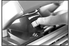
6. Rotate the power regulation knob to adjust the performance of the appliance.
