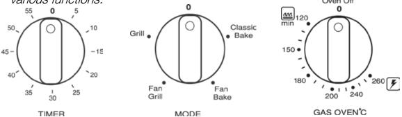
'TIMER': Minute counter – rotate the knob to the desired time up to 60 minutes and a bell will ring at the end of the time period. For very short time periods turn the knob past the point you want and then back to it to load the timer mechanism. Some models may have an electronic timer. Refer to electronic timer instructions in this book.
