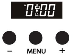
You need to set the timer before using your oven. It will flash on and off when you first connect the oven. This is normal.
