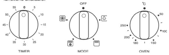
TIMER: Minute counter – rotate the knob to the desired time up to 60 minutes and a bell will ring at the end of the time period. For very short time periods turn the knob past the point you want and then back to it to load the timer mechanism. Some models may have an electronic timer. Refer to electronic timer instructions in this book.
