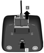
To disconnect the plug from the charger, press the release button 3 and disconnect the plug 4.
