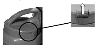
Next, rotate the top to unlock and pull the top from the dust canister.
