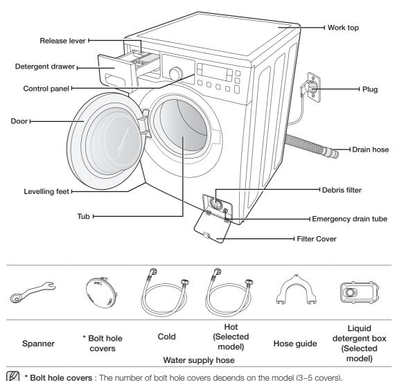
\* Bolt hole covers : The number of bolt hole covers depends on the model (3~5 covers).
