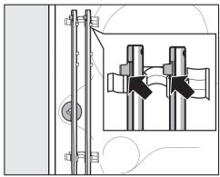
Secure the transit bars to the back of the washing machine. Make sure that the upper hooks are above the retainers.
