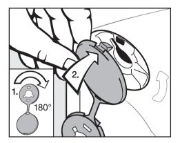
■ Fit the covers onto the two holes.
